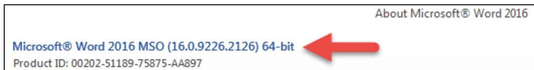
Figure 3 - About Word dialog. Note arrow pointing to information indicating this installation of Office is 64-bit.
